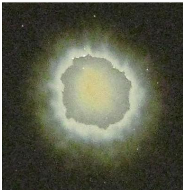
Far-field burn pattern of 1572 nm beam at 44 mJ
